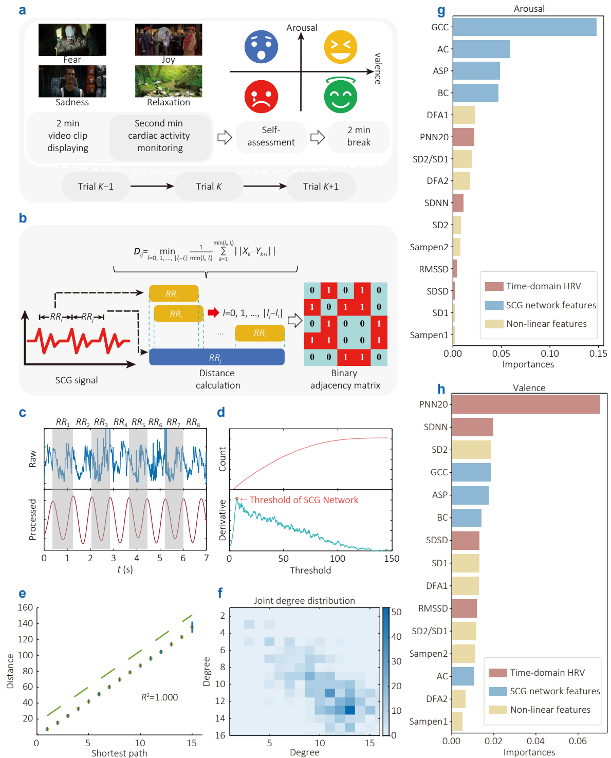
Fig. 3 | The experimental setup and feature engineering for emotion recognition. (a) Experimental setup for emotion recognition. (b) Construction method of the SCG network. Here, D denotes the adjacency matrix, l_i and l_j represent lengths of two intervals, X_k and Y_{k+l} refer to data points in the shorter and longer intervals, respectively. (c) RR intervals of the raw and processed SCG signal. (d) The method for selecting the binary threshold value. (e) Linear relationship between the shortest path in the SCG-binary network and the distances between RR intervals. (f) Joint degree distribution of the SCG network. Permutation importances of features in (g) arousal dimension and (h) valence dimension.
