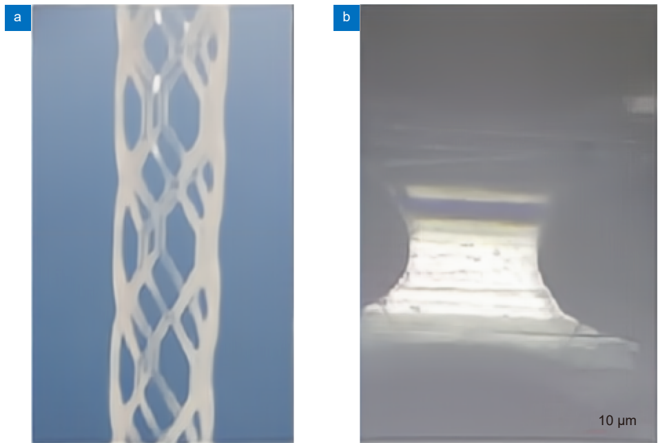
图 5 聚乳酸 (PLA) 激光加工 [21] 。(a) 支架结构; (b) 574 倍显微镜图 Fig. 5 Laser processing of PLA [21] . (a) Structure of PLA scaffold; (b) 574x micrograph
