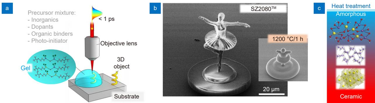
**Fig. 1 |** Top-down (a) and bottom-up (b) steps of nanomaterial synthesis. (c) Glass, crystalline, ceramic material is tuned via initial composition of a photo-curable precursor mixture and its thermal annealing at the required temperature, pressure, gas ambience. Surface tension driven reshaping is shown in scanning electron microscopy images in (b), where the same scale applies to both images before and after high temperature annealing.
