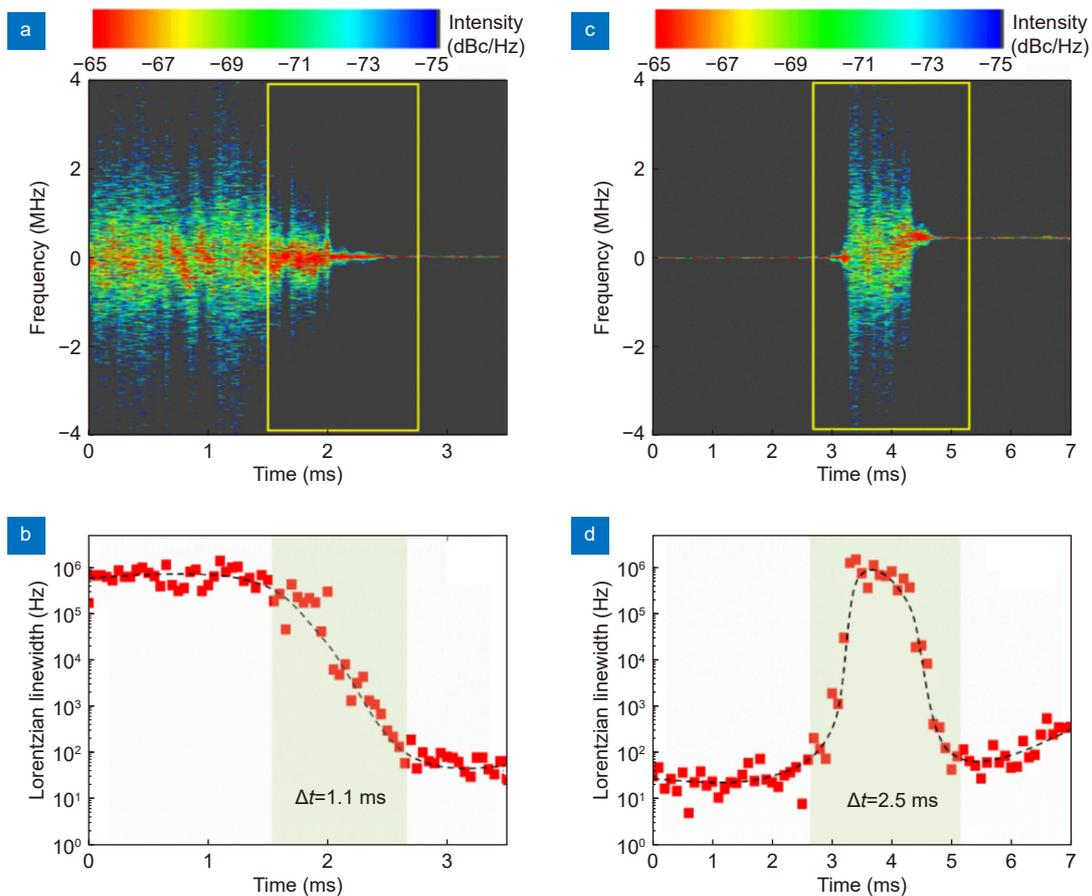
**Fig. 6 | Self-adaptive compression process of laser linewidth.** (a) Transient spectrum and (b) corresponding Lorentzian linewidth when switching on the feedback. (c) Transient spectrum and (d) corresponding Lorentzian linewidth when tuning the frequency of the main laser cavity.
