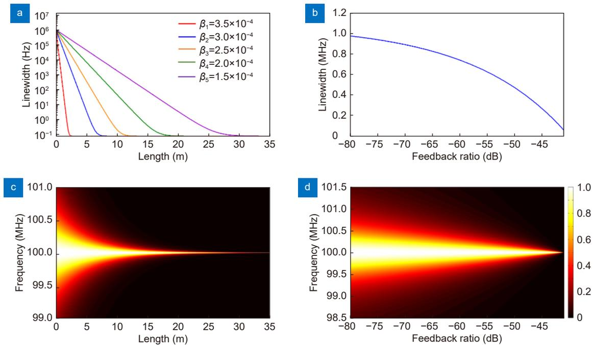
**Fig. 2 | Simulation results of laser linewidth evolution.** (a) Output linewidth evolution with the feedback length under different feedback coefficients. (b) Linewidth curve at the different feedback ratios. Two-dimensional pseudocolor maps of the spectra vary (c) with the length and (d) with feedback ratio.
