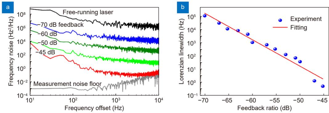
**Fig. 5 | Coherence of on-chip laser with different feedback ratios.** (a) Evolution curves of the frequency noise PSD under different feedback ratios. (b) Evolution curves of output linewidth with the feedback ratio.
