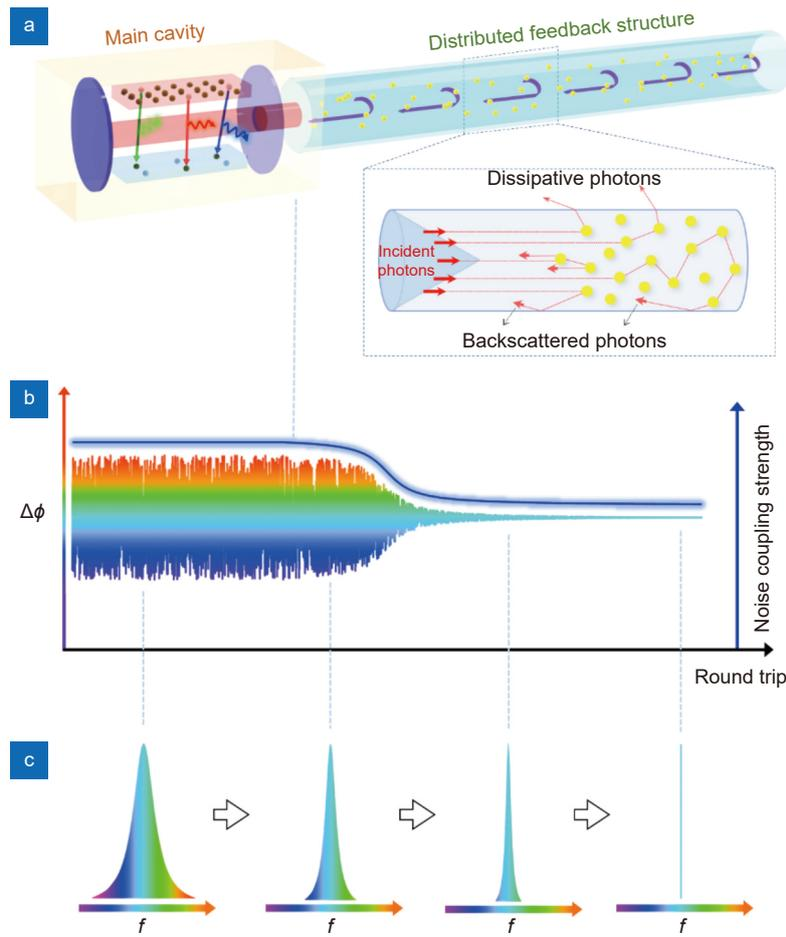
**Fig. 1 | Principle of laser spectral purification based on distributed weak perturbation.** (a) A novel laser configuration. (b) Evolution of laser phase fluctuation and noise coupling strength with different round trips. (c) Spectral distribution at different noise levels.
