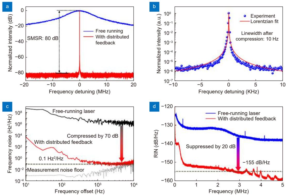
**Fig. 4 | Power spectra of the RF signal generated by beating two distributed feedback DFB lasers and spectral purity.** (a) Comparison curves of the frequency spectrum from beat frequency signal. (b) Lorentz fitting curve of the linewidth with a distributed feedback. (c) Comparison curves of the frequency noise PSD. (d) Comparison curves of the RIN spectrum, where a red curve indicates the compressed result.
