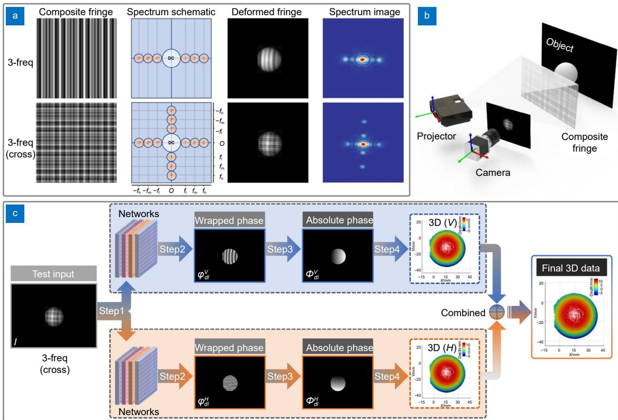
**Fig. 2 |** Possible future extension of the proposed DCFPP technique: (a) the example triple-frequency projected vertical and cross fringe patterns and their spectra, (b) the hardware system and (c) the enhanced shape reconstruction using cross fringe pattern and two channel reconstructions for vertical and horizontal composite fringe patterns.
