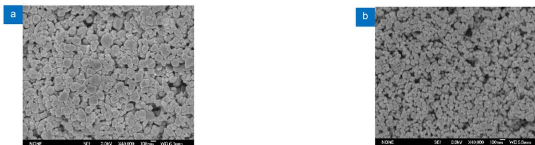
**Fig. 13 | SEM image of the ZnO nanoparticles fabricated by (a) doctor-blade method and (b) large scale ZnO film prepared by electro spray technique after heat treated at 460 °C for 1 h<sup>104</sup>.**
