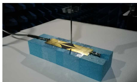
Fig. 9 | The photograph of the electromagnetic measurement system which is composed of a electromagnetic shielding chamber, a VNA and a monopole antenna (as a probe) installed in a mechanical platform which can scan the plane or space under the control of stepper motor.
