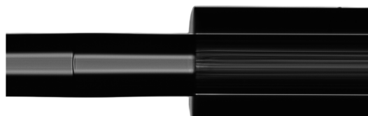
SMF-GRIN-HCARF after fusion splice
