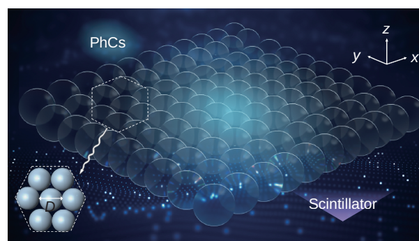
Fig. 1 | Schematic illustration of the self-assembled photonic crystal (PhC) scintillator. The device comprises a monolayer of polystyrene (PS) nanospheres self-assembled on a high-refractive-index GAGG:Ce scintillator. The central bright spot within the substrate indicates the scintillation process, where absorbed X-ray energy is converted into visible light emission. The unit cell composed of a hexagonal close-packed (HCP) lattice with a diameter ( D = 500 nm), inserted in the lower left corner, is periodically arranged along x- and y-directions to form a large diffraction grating.
