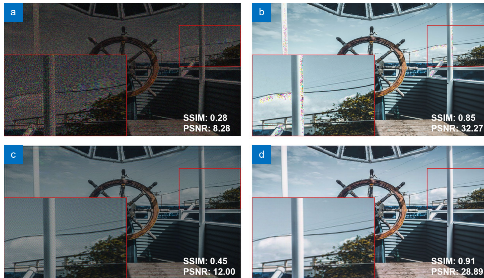
Fig. 3 | Comparisons of numerically reconstructed full-color images with conventional CGH methods with details magnification. (a) GS algorithm. (b) SGD algorithm. (c) DPAC algorithm. (d) IncepHoloRGB.
