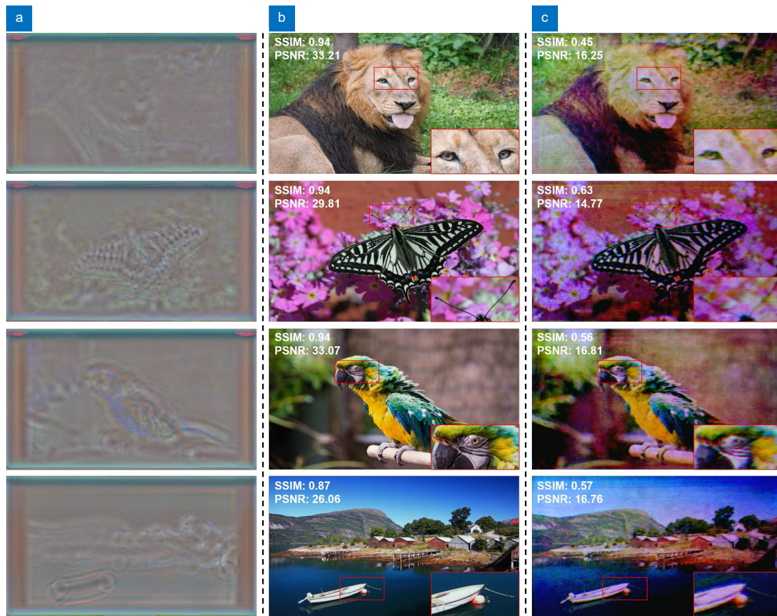
Fig. 4 | Holographic display of 2D scenes from IncepHoloRGB. (a) RGB POHs generated by IncepHoloRGB. (b) Numerically simulated reconstruction from (a) with details magnification in red boxes. (c) Optically experimental reconstruction from (a) with details magnification in red boxes.
