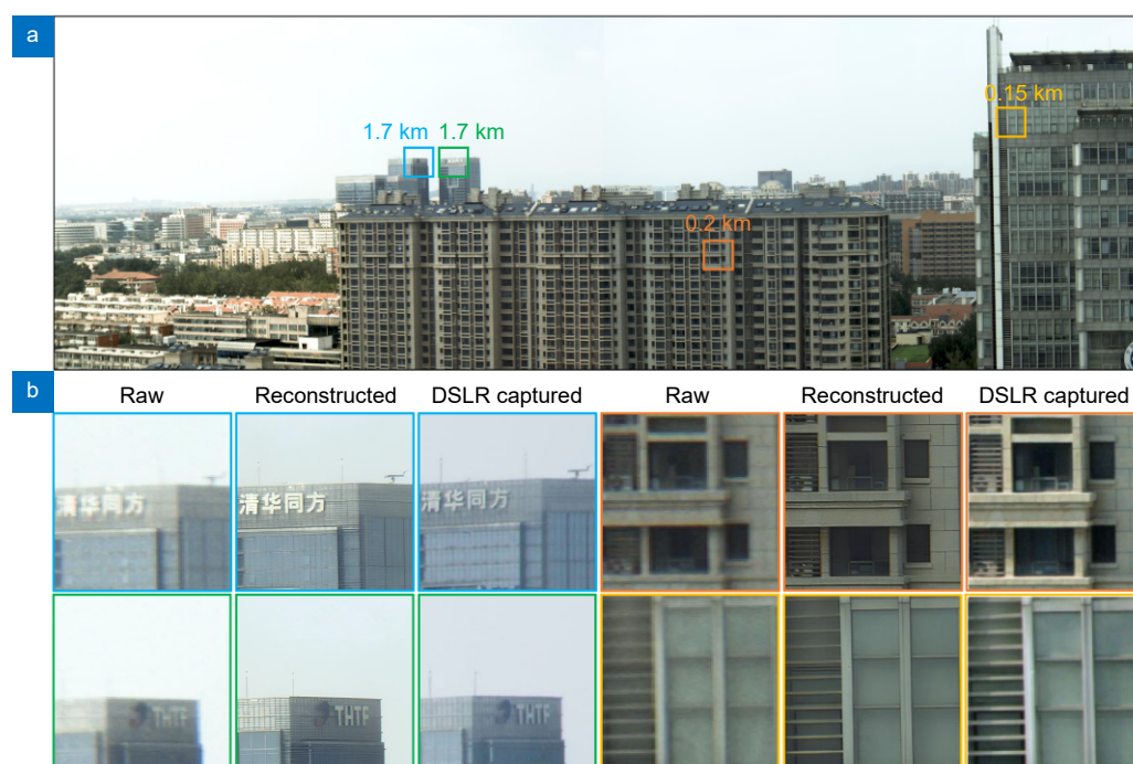
Fig. 5 | Imaging and high resolution reconstruction results of targets at different distances. (a) Large field of view image captured by the proposed sparse CEC. (b) Comparison between the raw images, reconstructed images through the dual-end collaborative zoom and optimization, and the images captured by a DSLR camera.
