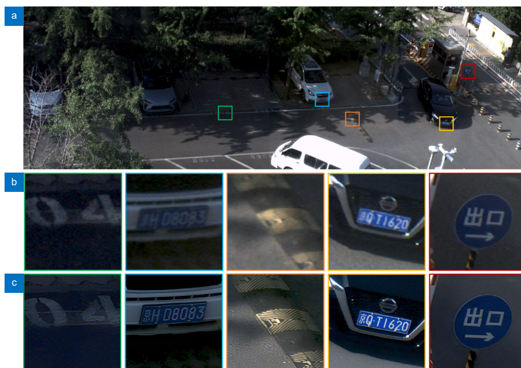
Fig. 4 | Imaging and high-fidelity reconstruction results for real scenes. (a) Large field of view image captured by the proposed sparse CEC. (b) Local magnification of the large field of view image. (c) Reconstructed high resolution images through the dual-end collaborative zoom and optimization.
