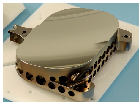
图 15 JSS-56 TMA 系统第三反射镜成品 [10] Fig. 15 Finished product of Jss-56 TMA system three mirror [10]
