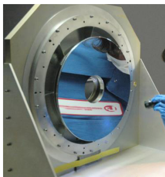
图 14 WISE 光学系统主镜实物图 [22] Fig. 14 Physical drawing of main mirror of wise optical system [22]
