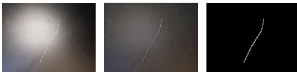
Pipeline defect visual inspection image processing
