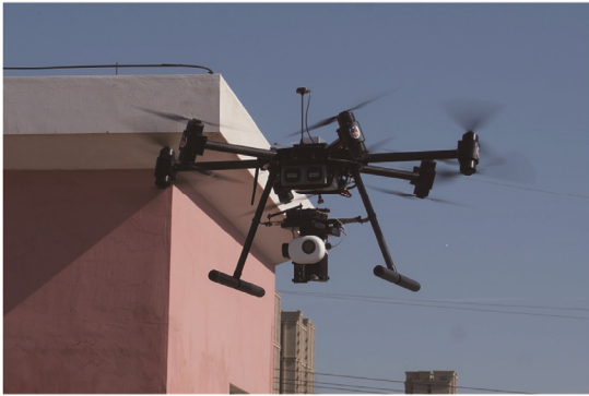
图 4 实验用搭载于多旋翼无人飞行器的机载光电平台。 Fig. 4 Airborne opto-electronic platform mounted on mUAV for experiment.
