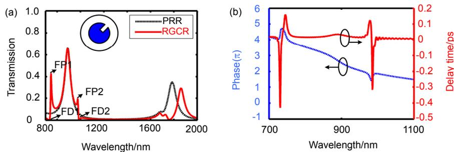
(a) Transmission spectra of PR resonator and RGCR structure with  $\varphi=90^\circ$  and  $L=100$  nm, and (b) phase response and delay time.
