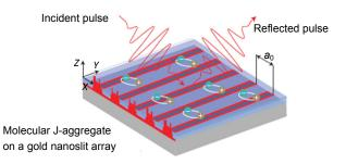
Schematic of coherent ultrafast spectroscopy on a hybrid nanostructure consisting of a 50-nm-thick film of J-aggregate molecules in a polymer matrix coated onto a gold nanogroove array with period  $a_0$ . Strongly localized SPP fields (in red) exist in and near the grooves. Incident and reflected laser pulses and J-aggregate excitons are shown schematically.
