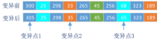
图4 遗传算法中染色体的变异过程 Fig. 4 Chromosome variation process in the genetic algorithm
